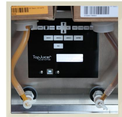
7. When the procedure is finish remove the bottles and reconnect the juice boxes to the unit. Once done, make on of each drink to ensure that the concentrate is pumped to the mixing system.
