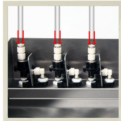
1. Disconnect the tubes by pressing the white plastic ring down against the metal ring and pull the tube out.
