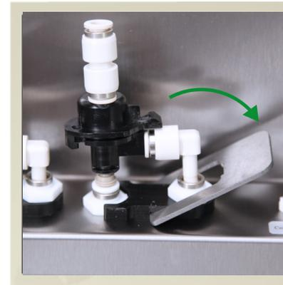
2. To gain access to the two connectors and the mixing unit, you have to tilt each metal plate to the right. Lift up in the mixing unit and the two connectors to release them. Do this for all 3 mixing units.
