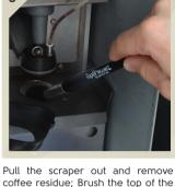
coffee residue; Brush the top of the brew unit using the brush with the long handle.
