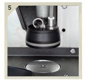
Wipe the top-plate with a damp cloth, pay special attention to the metal grate on the bottom piston. Wipe the underside and inside of the scraper. Check the stainless steel bottom-piston head is clean and without coffee residue. Push the scraper back in
