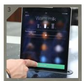
Slide the number of cups up to 5 and select "Start now". The machine will run the cleaning liquid through the system and clean the milk foamer.
