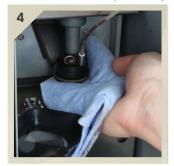
Wipe throughly beneath the toppiston, so that the metal filter, o-ring and the area around is clean. This prolonges the brewers lifetime.
