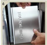
Take out the dregbin, and empty the coffeegroundbag. Clean and wipe the bin before replacing the bag. Remember the machine resets the counter each time the bin is removed. Therefore if should always be emptied if taken out.
